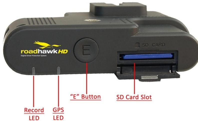
**Record LED:** Will light red when the camera is recording normal video. It will flash red when the camera is recording an EVENT.
