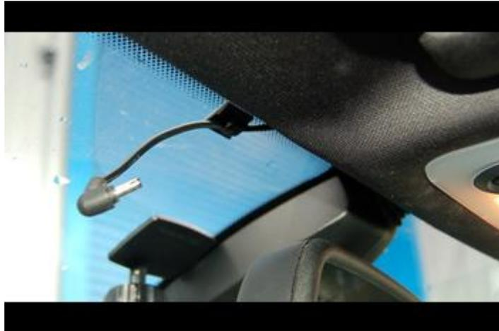
**6:** Run the cable around the side of the dashboard and underneath towards the cigarette lighter socket. Use the cable ties to hide any remaining cable behind the dash.
